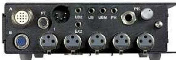
The essential information for connecting to and operating the mixer is permanently printed on the baseplate.
