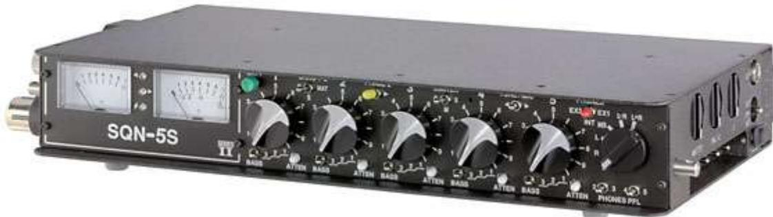
The new SQN-5S Series II expands upon the virtues of its predecessor, including transformerless input and output amplifiers for reduced weight and uninhibited bass, virtually unbreakable analogue level meters, four channels of pre-fade listening, slating microphone, superb limiter, output feed for all five microphone channels and logic processing of most switching giving a minimal length audio path.
