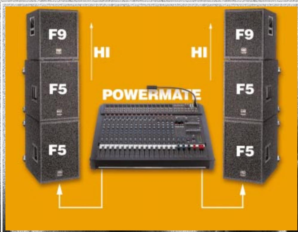
The Xa5 loudspeaker system can also be used without a problem in passive system configuration employing the F5's passive frequency crossover. And again, the wiring is reasonably easy: The power mixer's power outputs have to be connected to the lower F5 cabinet. From here cabling leads to the upper F5 sub woofer system and through utilizing its crossover output, the F9CWH cabinet gets connected.
